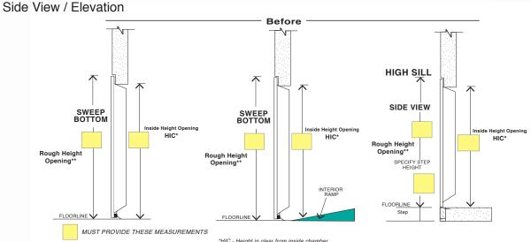
\*\*Rough Height Opening - Height of opening from outside of chamber
