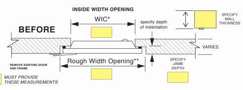
\*WIC - Width in clear from inside chamber \*\*Rough Width Opening - Width of opening from outside of chamber It is critical that we get the opening size (interior, exterior and wall thickness), not just door measurements.
