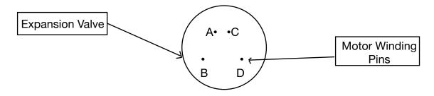
For valve size 29320003 and 2930004, the resistance measured between pin locations A and B or C and D should be approximately 336 Ohms when valve is at 75°F.
